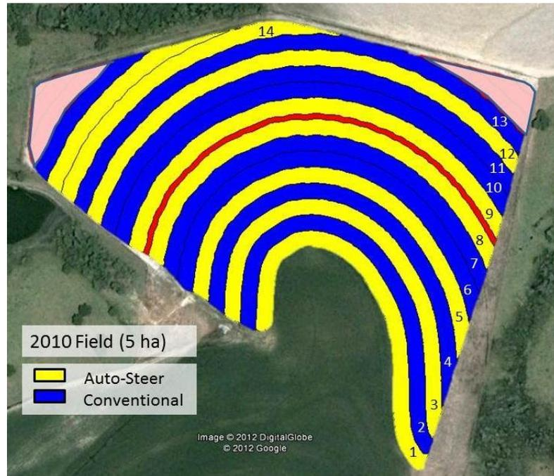
Figure 2. Experimental design used in 2010. Each replicate (colored strip) = 12 rows of peanuts or three 4-row passes
