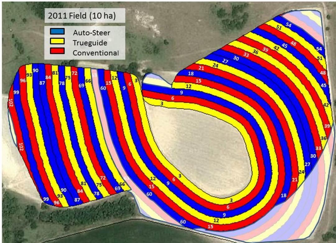
Figure 3. Experimental design used in 2011. Each replicate (colored strip) = 12 rows of peanuts or three 4-row passes
