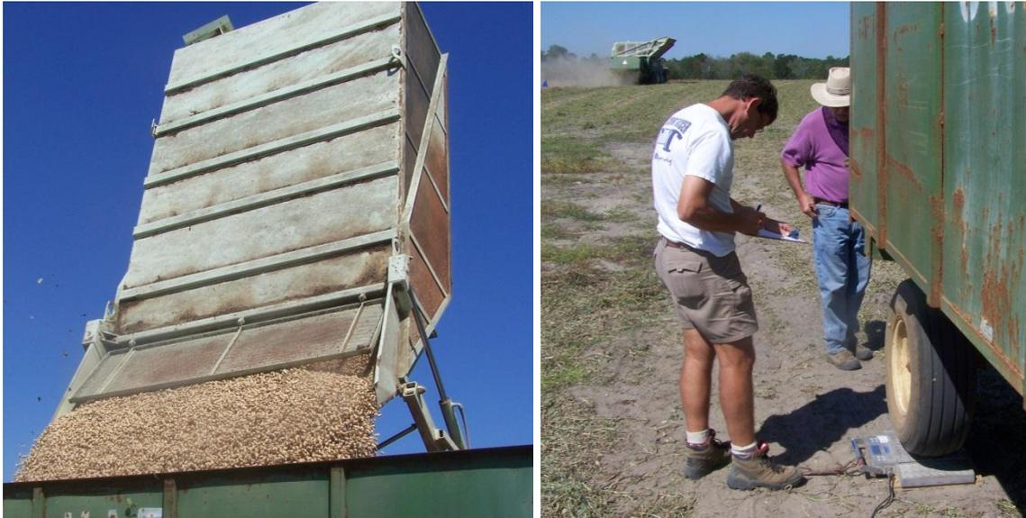
Figure 5. Peanut harvester emptying a load of peanuts into a peanut wagon (left) and load scales used to record weight of peanuts harvested from a pass (right). A load scale is located under each wheel of the wagon.
