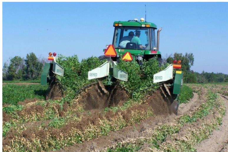
Figure 4. Inverting peanuts with a 4-row KMC peanut inverter pulled by the UGA tractor equipped with a Trimble® AgGPS Autopilot™ auto-steer system.
