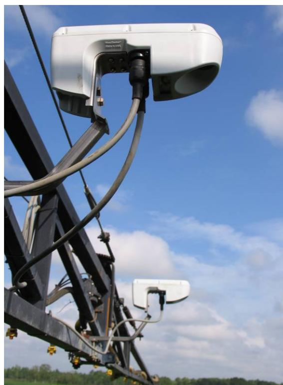
Figure 2. Two of the 6 GreenSeeker<sup>®</sup> sensors mounted on the spray boom of the JD6700 high clearance sprayer used in the study.
