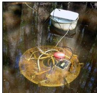
Figure 2. SOD chamber with datalogging computer
