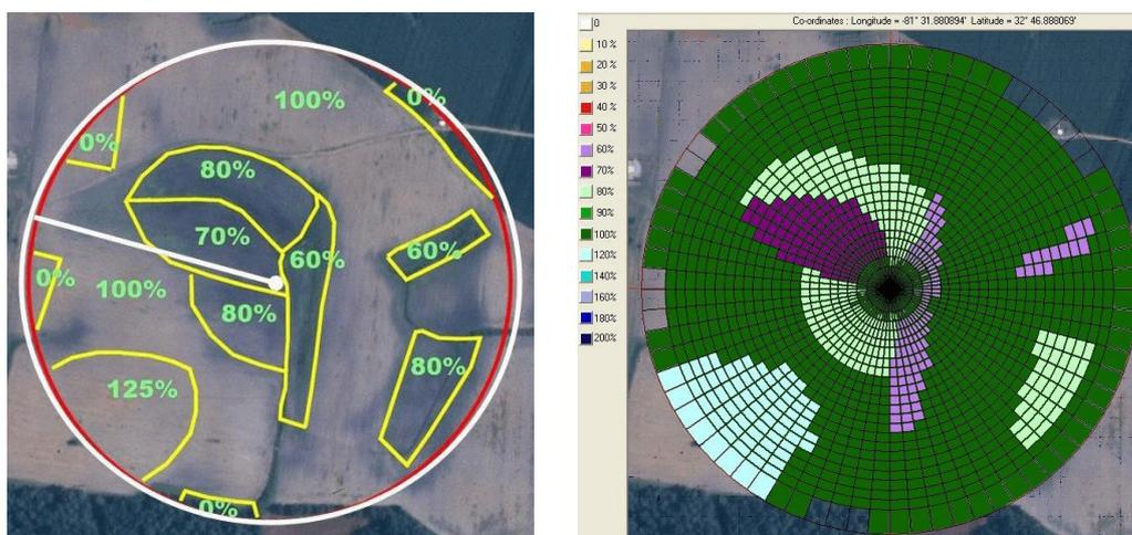
Figure 3. Irrigation application rates assigned to different areas under a 48 ha center pivot irrigation system (left) and VRI implementation of the application map (right).
