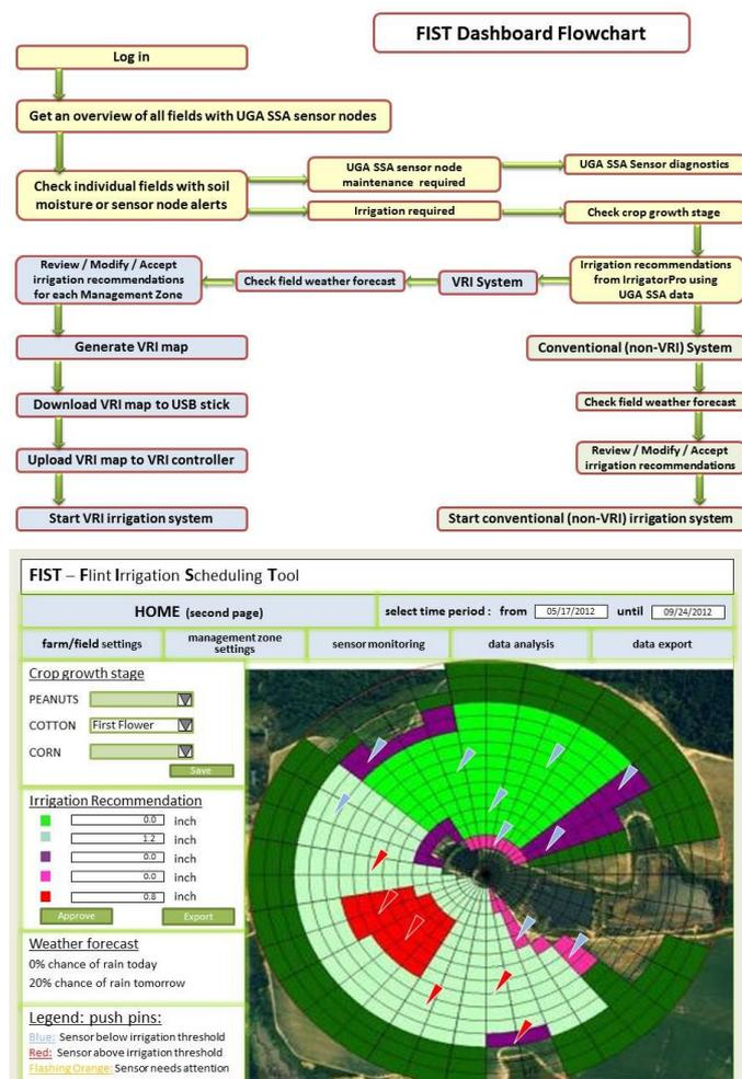
Figure 4. FIST flow diagram (top) and FIST dashboard (bottom).
