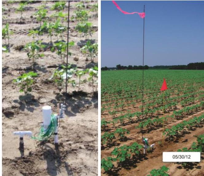
Figure 2. To increase transmittance range and to allow for farm vehicles to pass over the node, the electronics are kept at the soil surface and the antenna enclosed in a 2.5 m, 60 mm diameter hollow, flexible, spring-loaded fiberglass rod.
